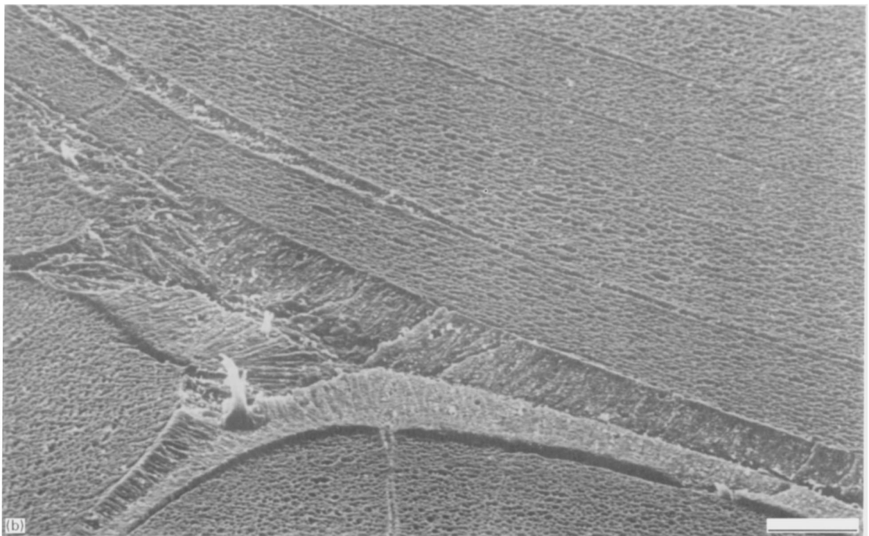
Figure 8 (a) An etched section through a sample compacted at 178°C (scale bar = 10 μm). (b) An etched section through a sample compacted at 182°C (scale bar = 10 μm).
